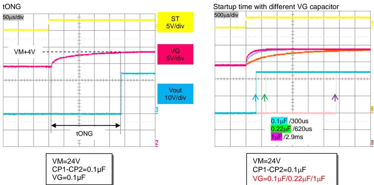
Figure 47. VG voltage pressure waveform
