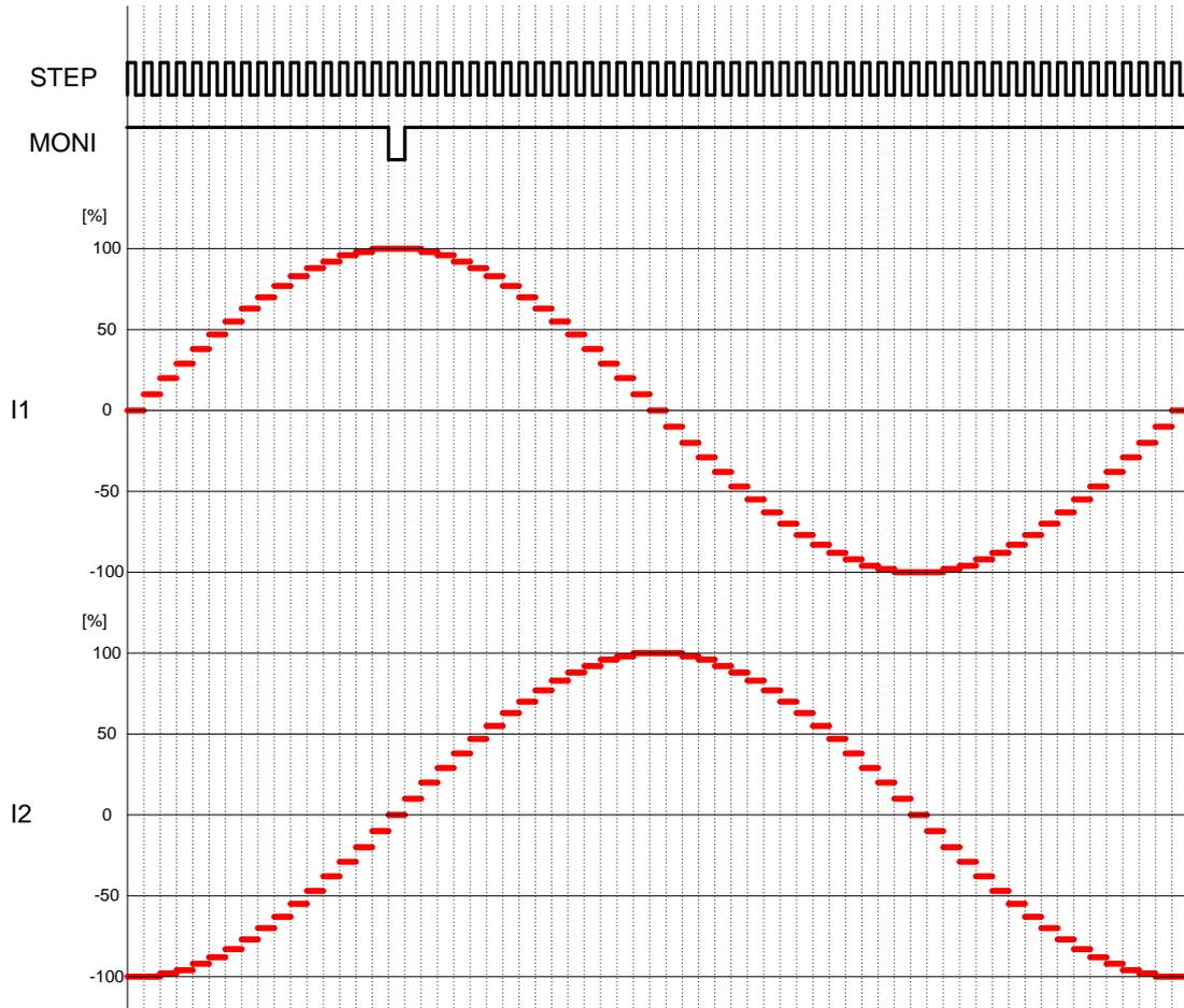
Figure 26. Current waveform of 1/16 step in CLK-IN
