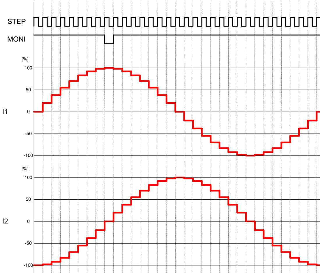
Figure 25. Current waveform of 1/8 step in CLK-IN
