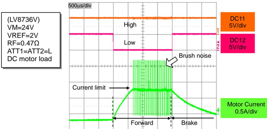
Figure 36. Current limit operation
