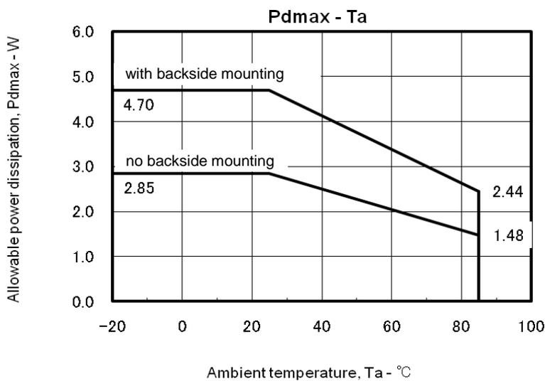
**Substrate Specifications** (Substrate recommended for operation of LV873XV)
