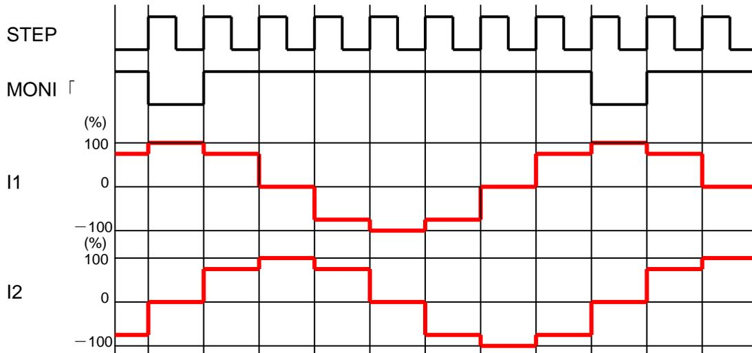
Figure 23. Current waveform of Half step in CLK-IN
