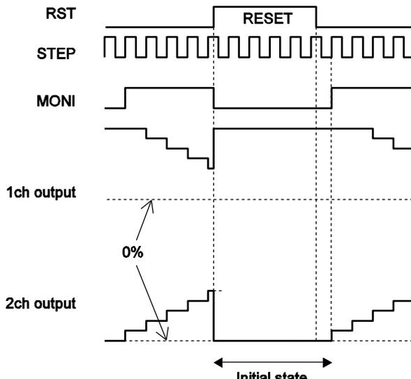
Figure 18. Reset operation
