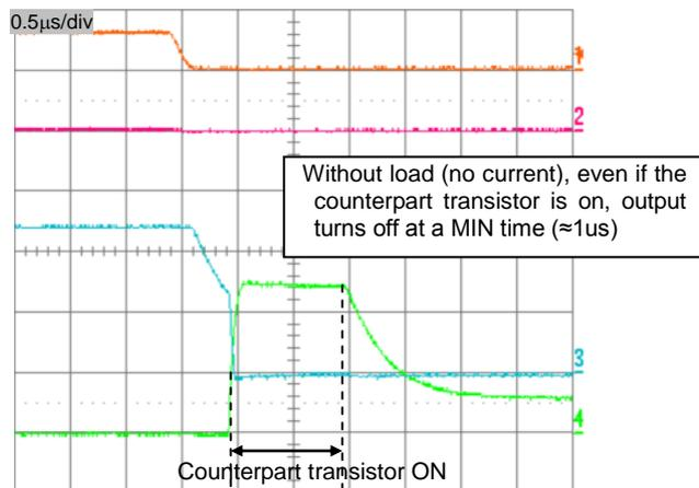
Coil load VM=24V, DC11=10kHz (DC12=L)
