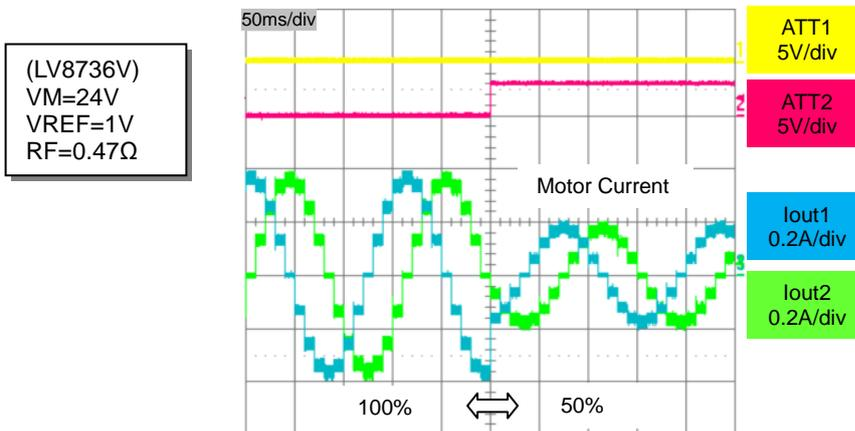
Figure 17. Attenuation operation
