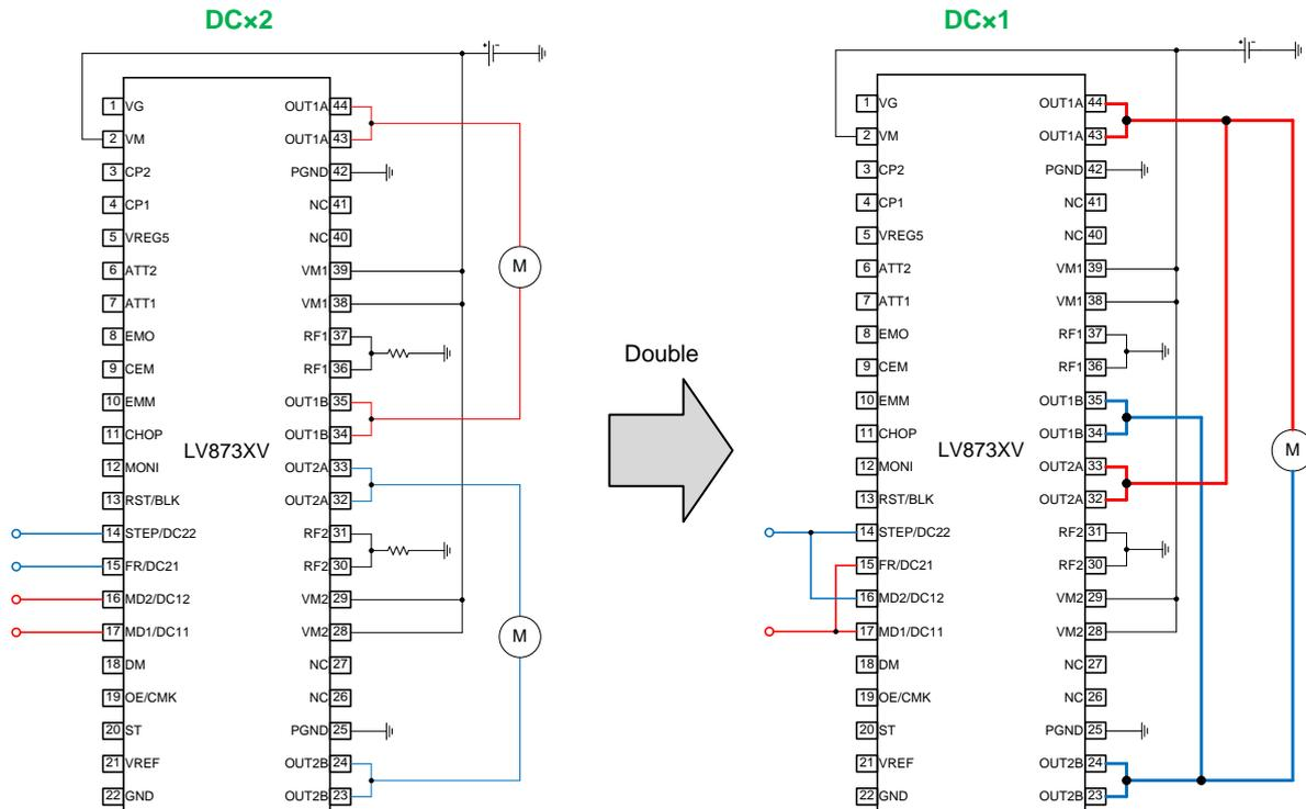
Figure 40. Parallel connection at DCM
