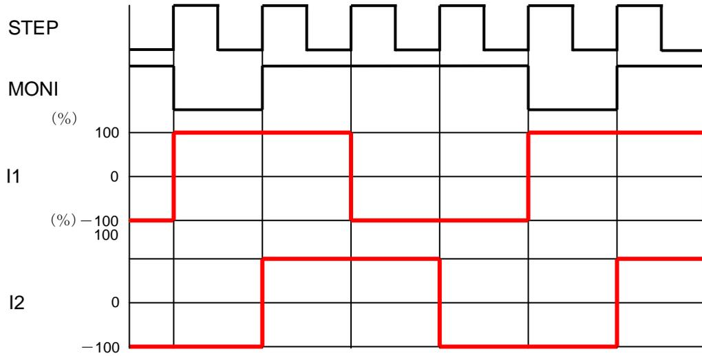
Figure 22. Current waveform of Full step in CLK-IN
