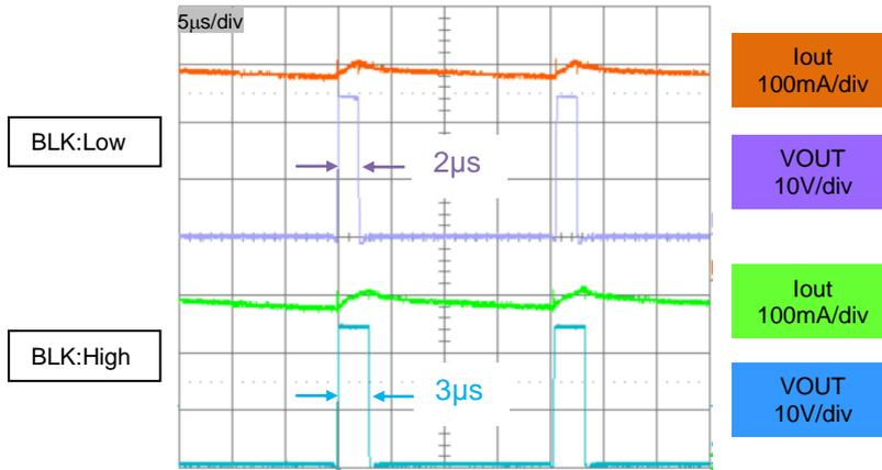
Figure 39. Blanking time waveform
