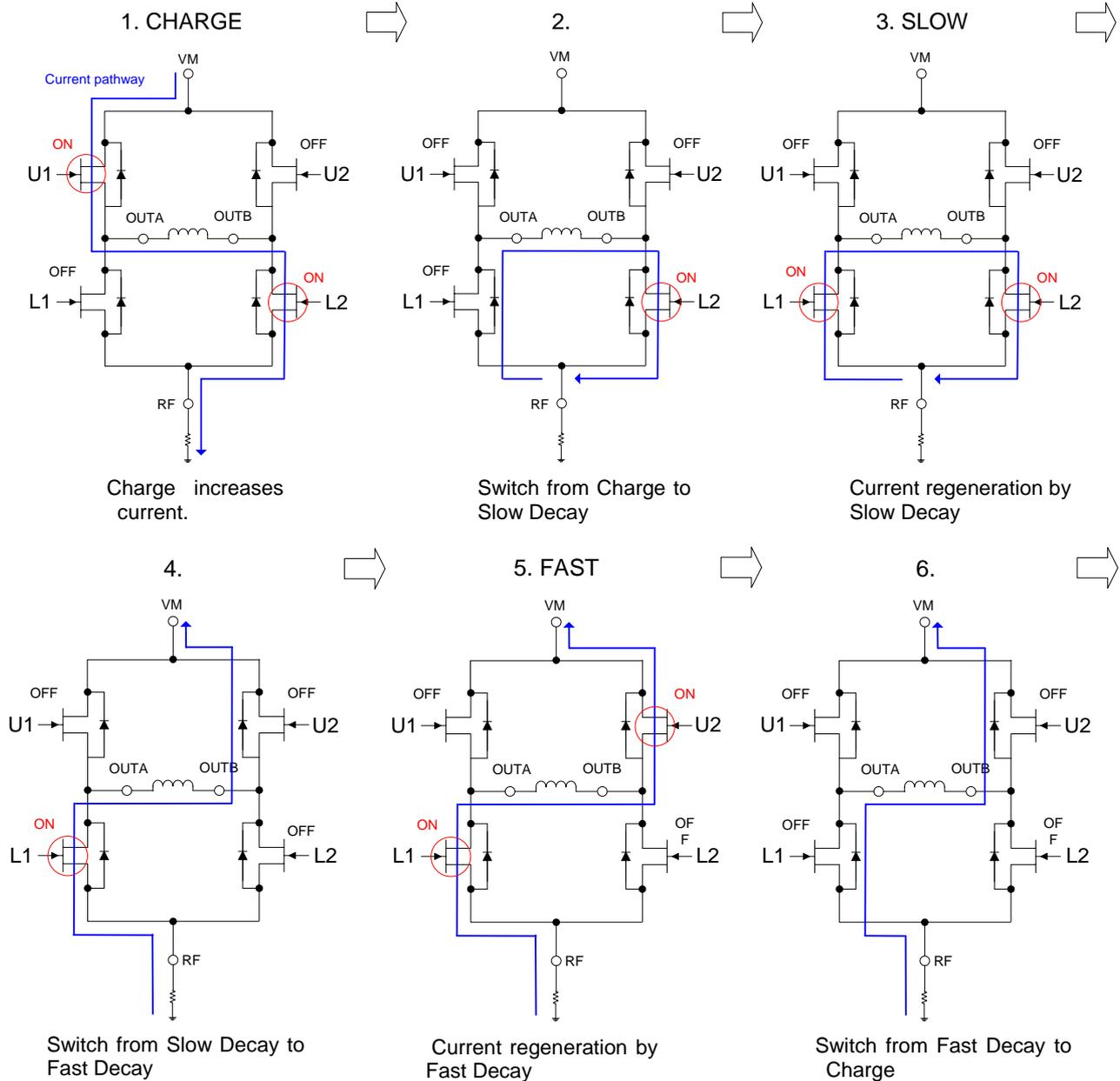
Figure 28. Switching operation
