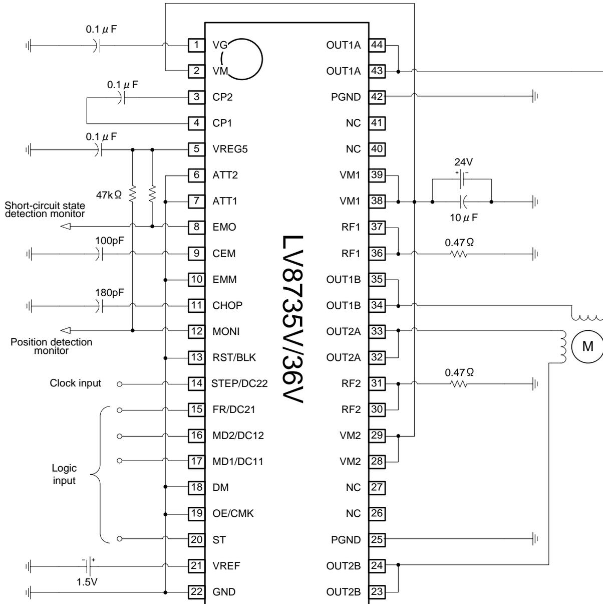
The formula for setting the constants in the examples of the application circuits above are as follows :
