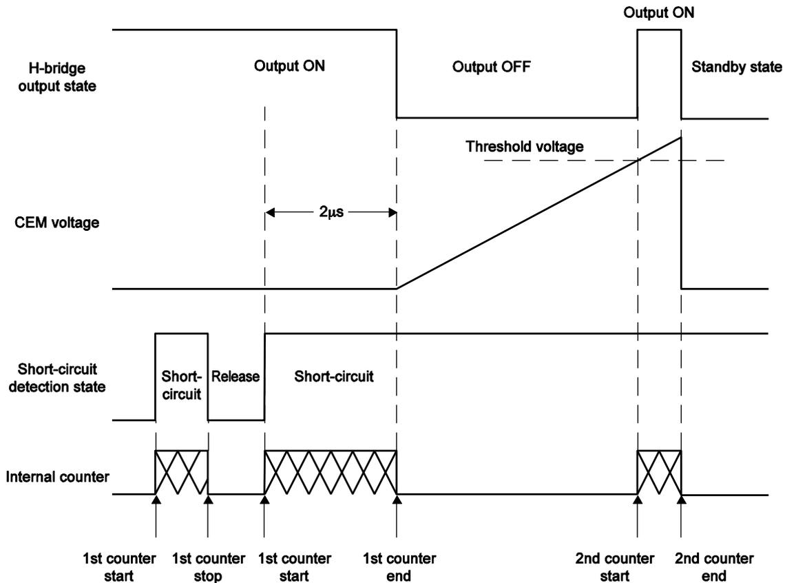
Figure 44. CEM operation timing chart in latch type
