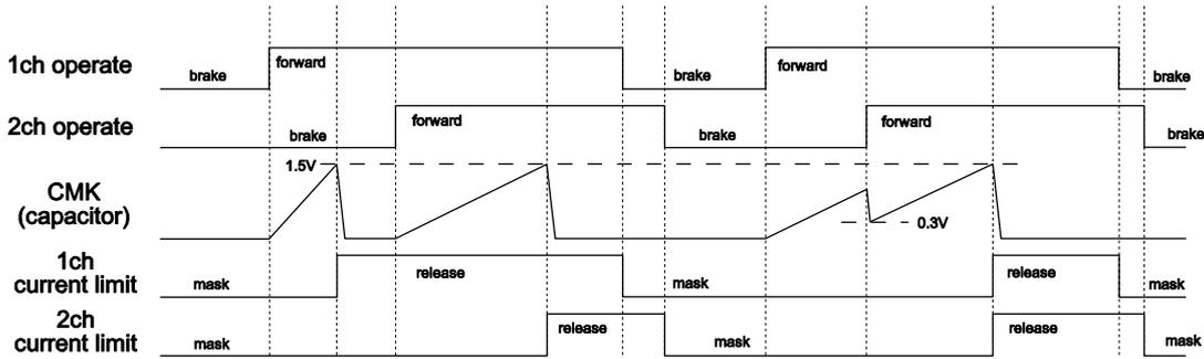
Figure 37. Current limit mask function timing chart
