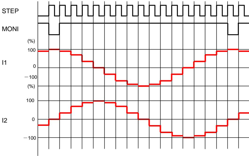
Figure 24. Current waveform of Quarter step in CLK-IN
