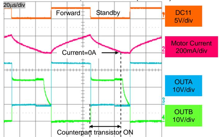
Standby mode turns on the counterpart transistor
