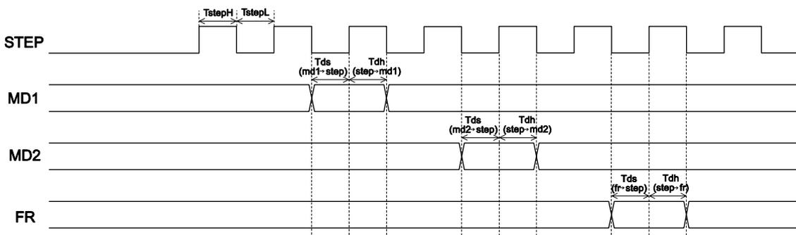
TstepH/TstepL : Clock H/L pulse width (min 500ns)
