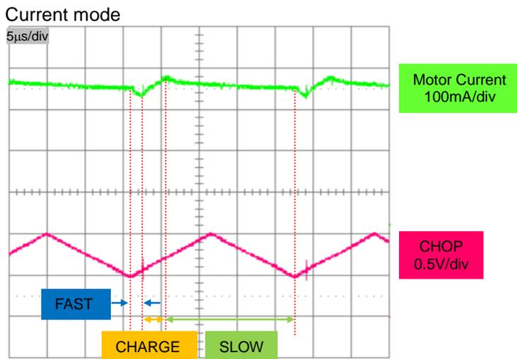
Figure 30. Chopping waveform
