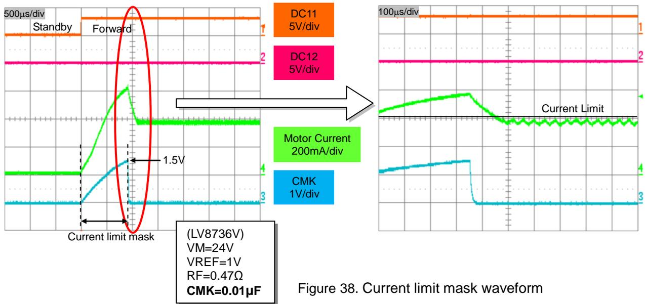
Figure 38. Current limit mask waveform
