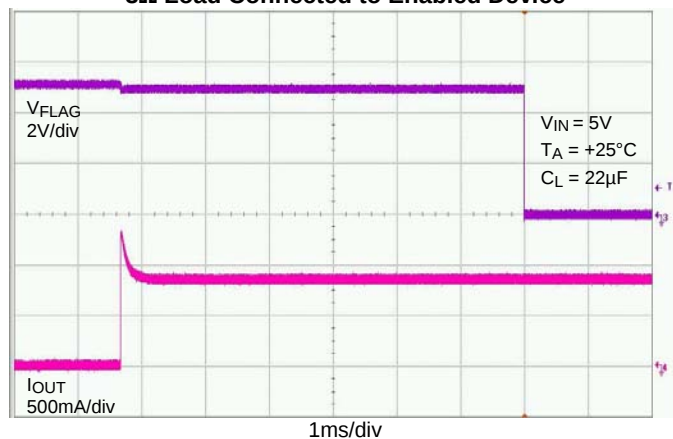
3Ω Load Connected to Enabled Device
