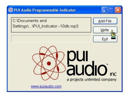
6. The software will erase any previously written file and write the selected file into the indicator. The status window will show "SPI programming". This only takes a few seconds.
