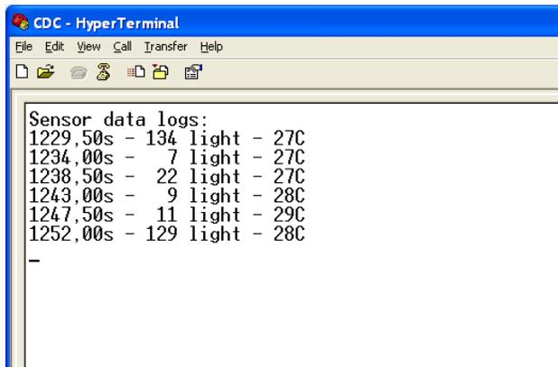
Note: The Virtual COM port is not connected to a true RS232 COM port, thus the baudrate and parity parameters can be ignored.
