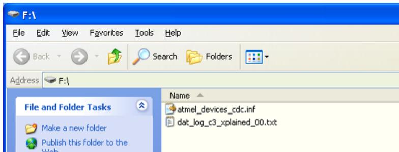
The CDC interface uses the native driver from UNIX® O.S., but requires a specific one on Windows® O.S. When the USB feature is disabled, the Windows driver file is created by demo application on the microSD card. After USB MSC startup or through another SD card reader, the `atmel_devices_cdc.inf` file can be selected to install the new USB CDC interface.
