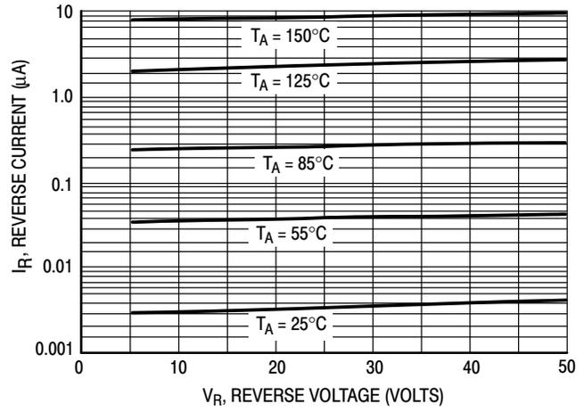
**Figure 5. Leakage Current**
