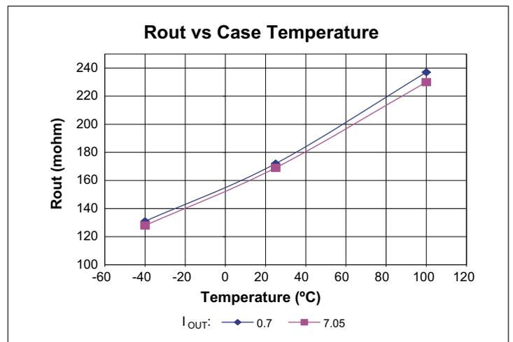
Figure 6 —  $R_{OUT}$  vs. temperature vs.  $I_{OUT}$
