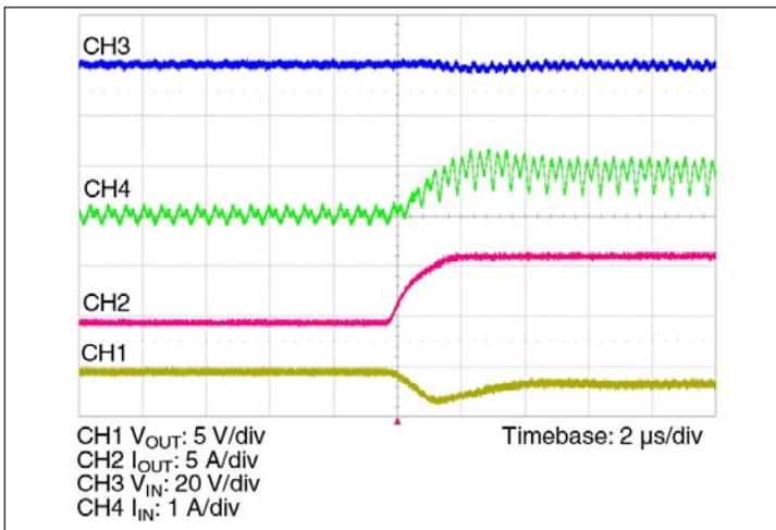
Figure 11 — Positive load transient (0 – 7.07 A)
