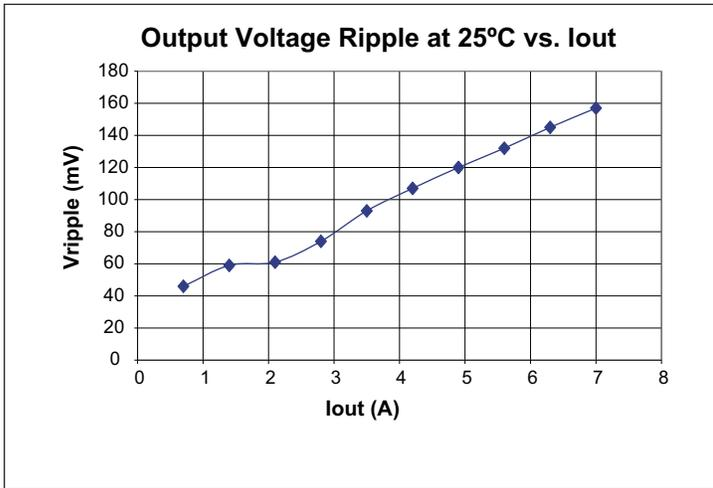
Figure 7 — Vripple vs. I<sub>OUT</sub>; 384 V<sub>IN</sub>, no external capacitance
