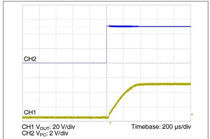
Figure 8 — PC to V<sub>OUT</sub> start up waveform
