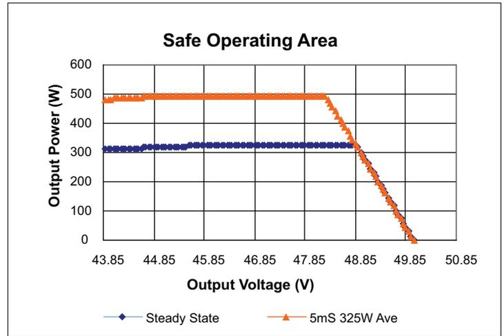
Figure 14 — Safe Operating Area vs. V<sub>OUT</sub>
