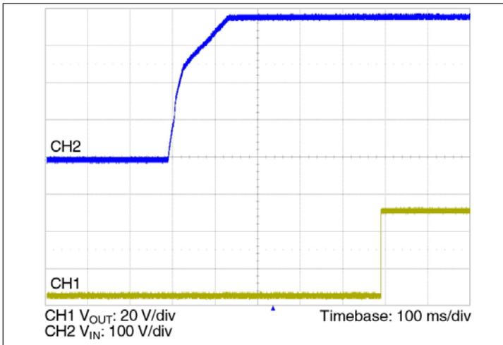
Figure 9 — V<sub>IN</sub> to V<sub>OUT</sub> start up waveform
