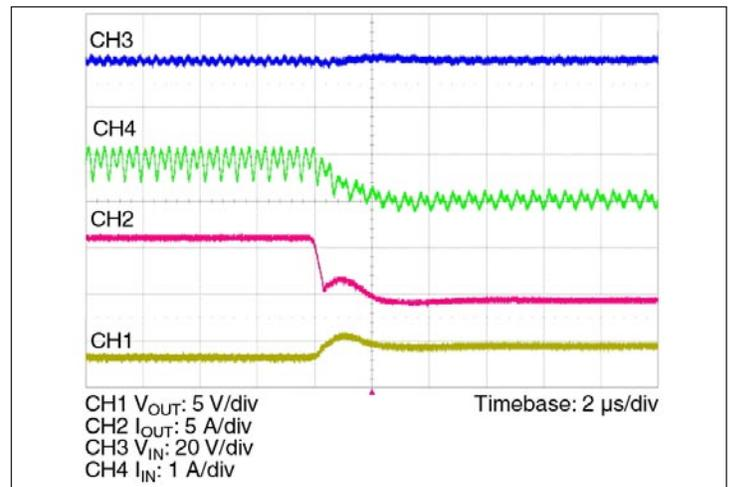
Figure 12 — Negative load transient (7.07 A – 0 A)
