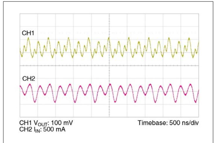
Figure 10 — Output voltage and input current ripple, 384 V<sub>IN</sub>, 325 W no C<sub>OUT</sub>
