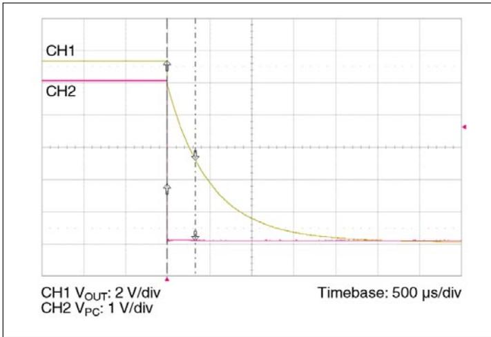
Figure 13 — PC disable waveform, 384 V<sub>IN</sub>, 100 μF C<sub>OUT</sub> full load
