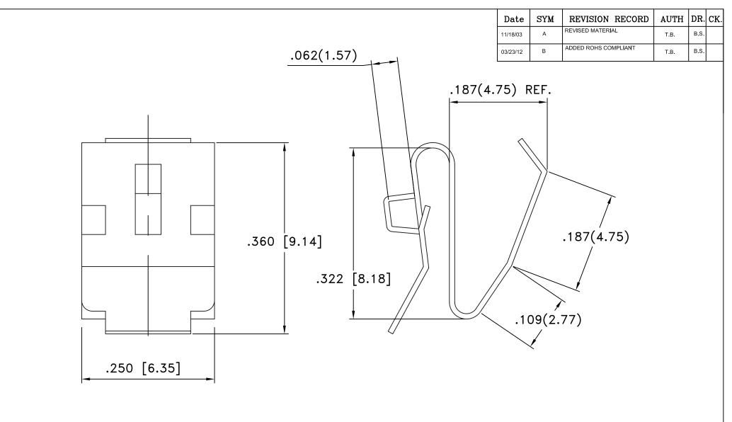
MATERIAL: 0.010" SPRING TEMPER STAINLESS STEEL, NICKEL PLATED ROHS COMPLIANT
