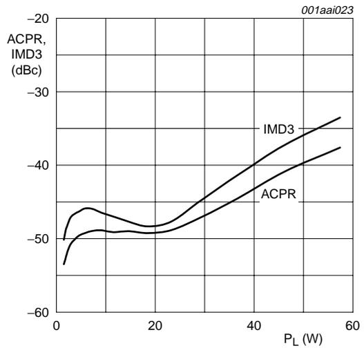
$V_{DS} = 32$  V;  $I_{DQ} = 1600$  mA;  $f_1 = 1867.5$  MHz;  $f_2 = 1877.5$  MHz; carrier spacing 10 MHz.
