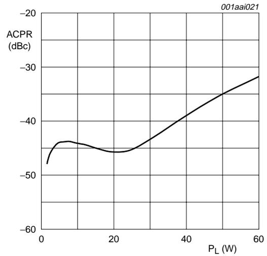
$V_{DS} = 32$  V;  $I_{DQ} = 1600$  mA;  $f_1 = 1872.5$  MHz;  $f_2 = 1877.5$  MHz; carrier spacing 5 MHz.
