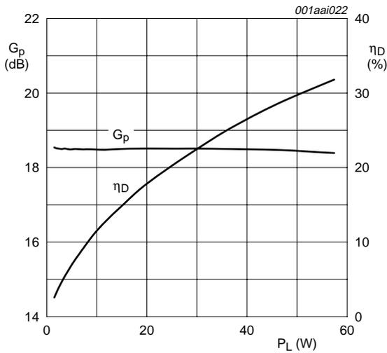
$V_{DS} = 32$  V;  $I_{DQ} = 1600$  mA;  $f_1 = 1867.5$  MHz;  $f_2 = 1877.5$  MHz; carrier spacing 10 MHz.
