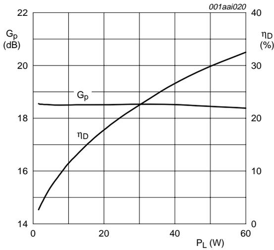
$V_{DS} = 32$  V;  $I_{DQ} = 1600$  mA;  $f_1 = 1872.5$  MHz;  $f_2 = 1877.5$  MHz; carrier spacing 5 MHz.
