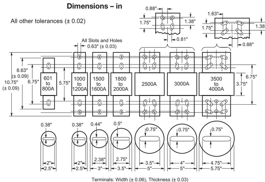
**Description:** Advanced protection Class L time-delay, current-limiting fuses. Time-delay – 5 seconds (minimum) at 500% of rated current.
