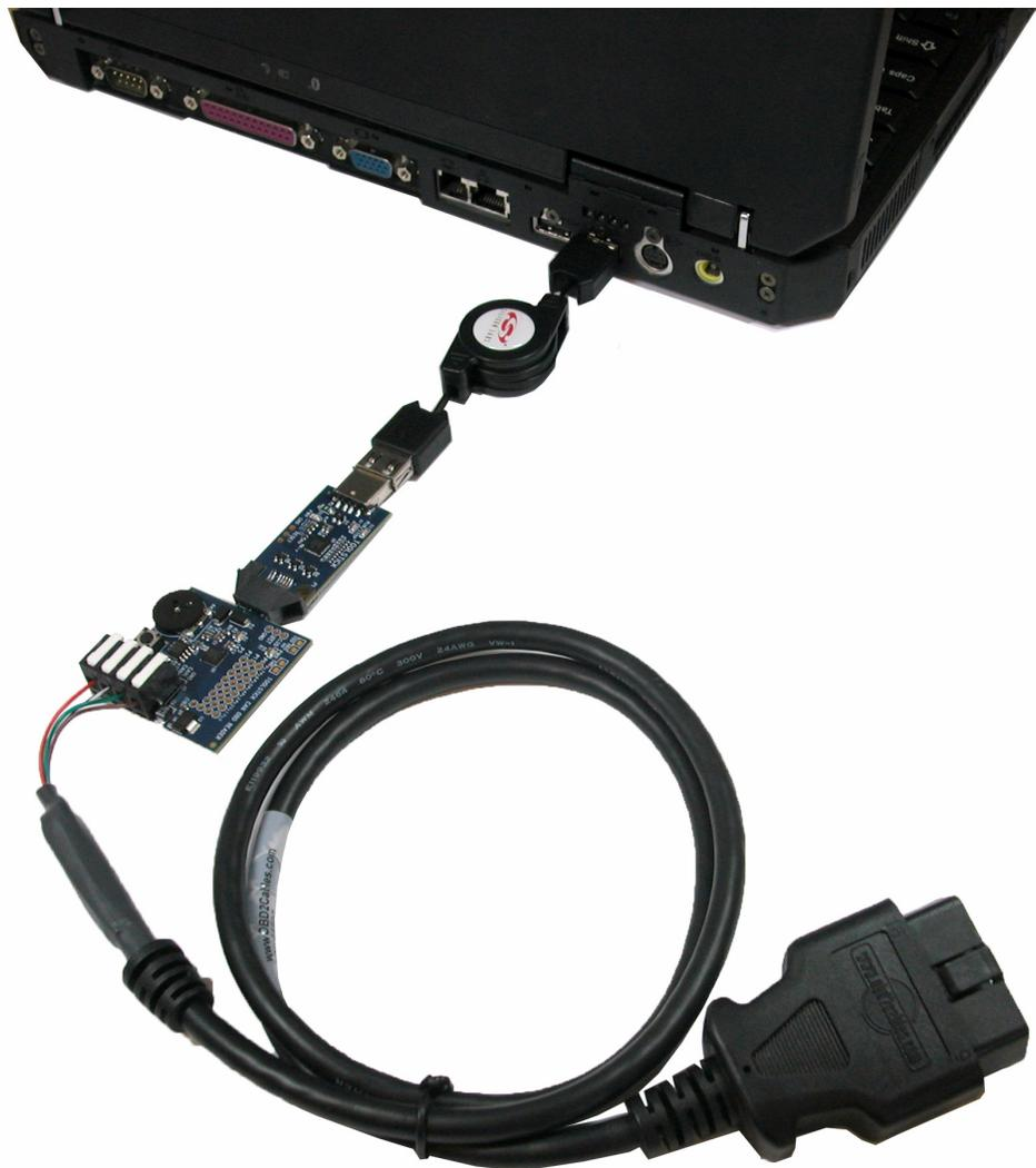
**Figure 5. OBD Reader Connected to the PC**
