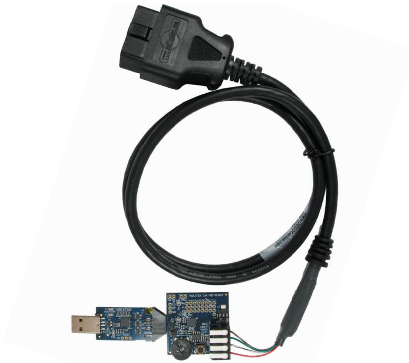
Figure 3. CAN OBD Reference Design Hardware
