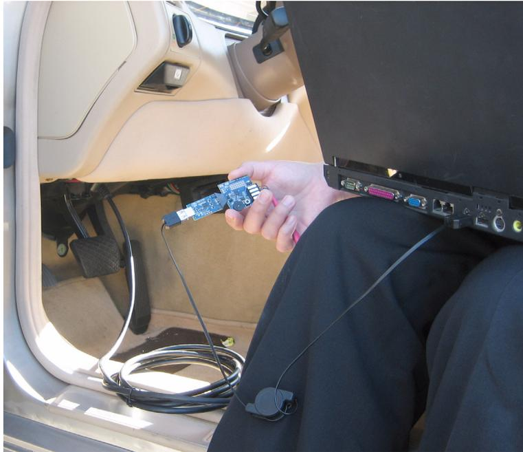
**Figure 9. Real-Time Mode Hardware Setup**
