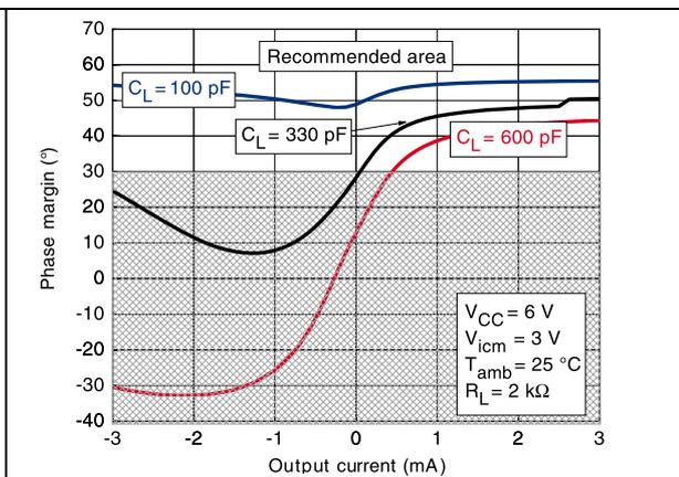
**Figure 20. Phase margin vs. output current, at  $V_{CC} = 10\text{ V}$ ,  $V_{icm} = 5\text{ V}$  and  $T = 25\text{ }^\circ\text{C}$**
