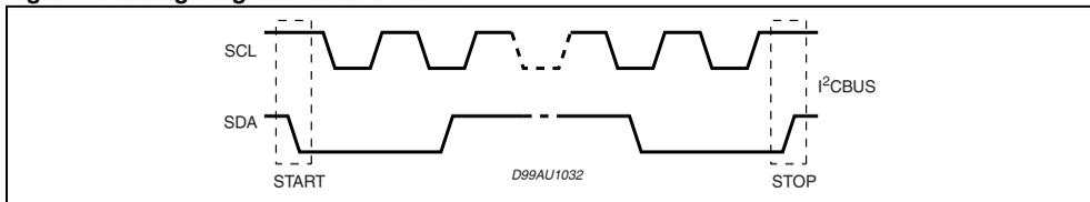
Figure 4. Acknowledge on the I<sup>2</sup>C Bus
