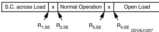
$$R_{1,SE} = \frac{L_{SC,max}}{I_{source}} = \frac{L_{SC,max}}{54.45} \cdot R_{CS}$$
