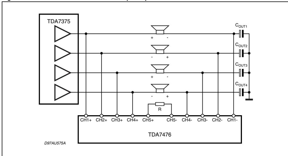
Figure 8. TDA7375 in S.E. mode with 2 output capacitors
