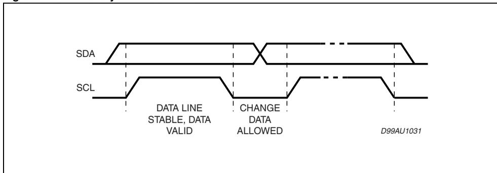
Figure 3. Timing Diagram on the I<sup>2</sup>C Bus
