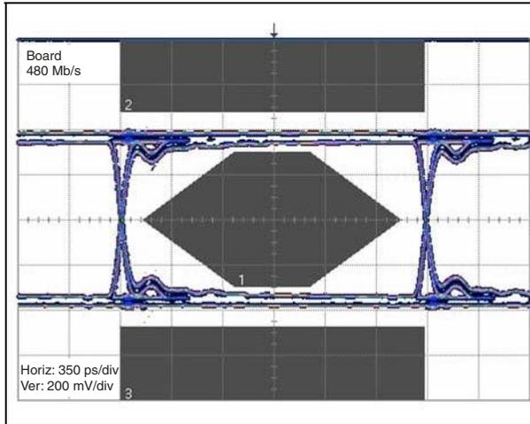
Figure 4. Eye diagram, board with USBULC6-2F3 (according to USB 2.0 high speed specification)
