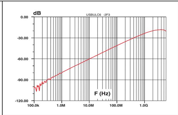
Figure 11. S21 (dB) attenuation measurement
