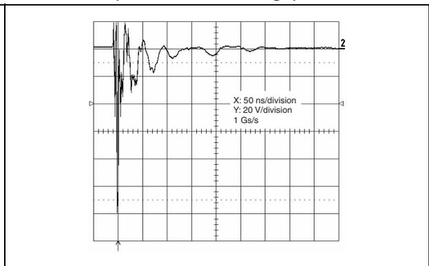
Figure 7. ESD response to IEC 61000-4-2 (+8 kV contact discharge)<sup>(1)</sup>
