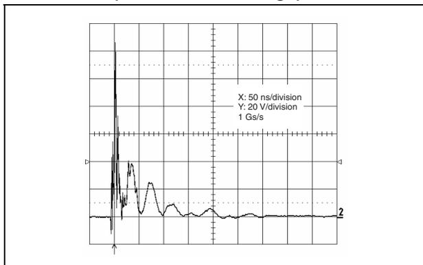
Figure 6. ESD response to IEC 61000-4-2 (-15 kV air discharge)
