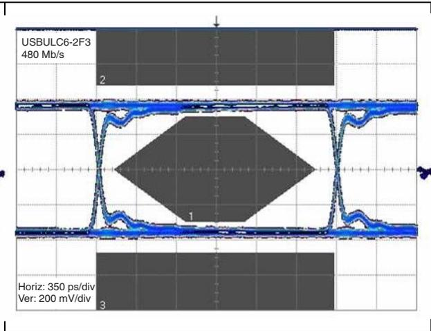
Figure 5. ESD response to IEC 61000-4-2 (+15 kV air discharge)
