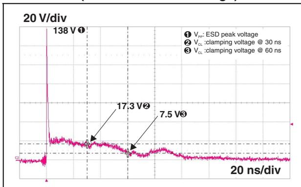
Figure 8. ESD response to IEC 61000-4-2 (-8 kV contact discharge)<sup>(1)</sup>
