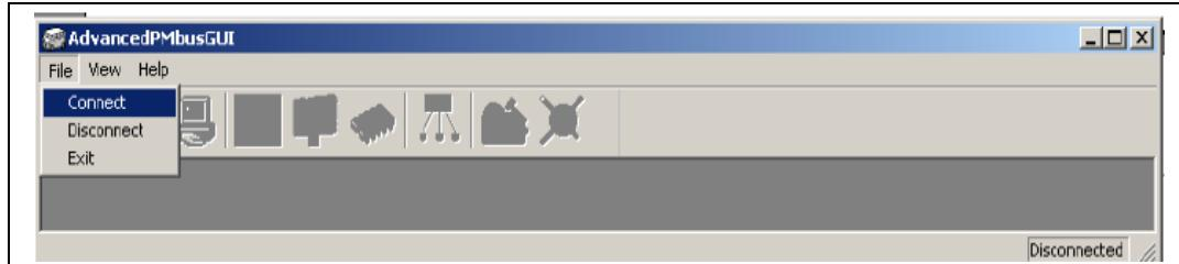
If the demonstration board is connected to the PC GUI, it shows 'Connected' in the status bar (on the bottom right-hand of the GUI screen) and the device selection window appears.
