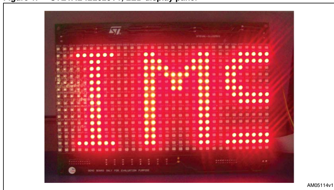
Figure 1. STEVAL-ILL025V1, LED display panel
