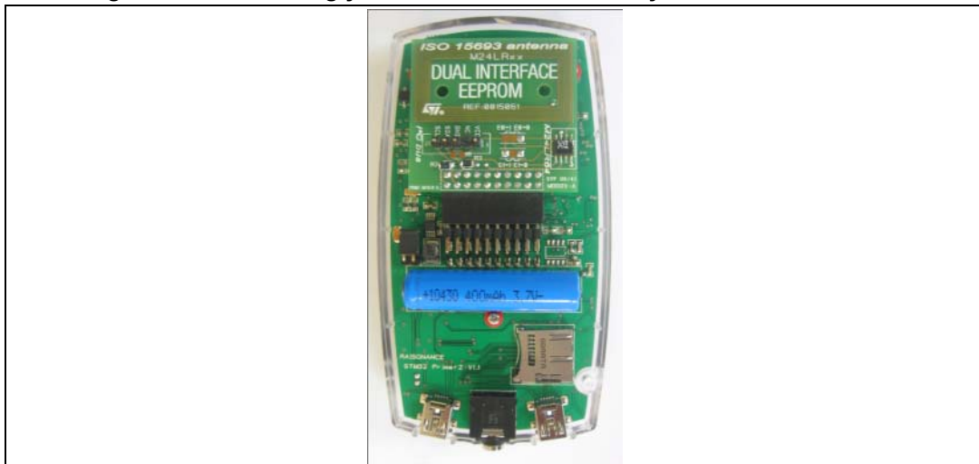
Figure 50. Connecting your reference antenna to your STM32-PRIMER2
