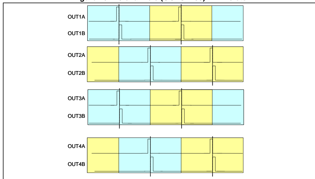
Figure 16. 2.0 channels (OCFG = 00) PWM slots
