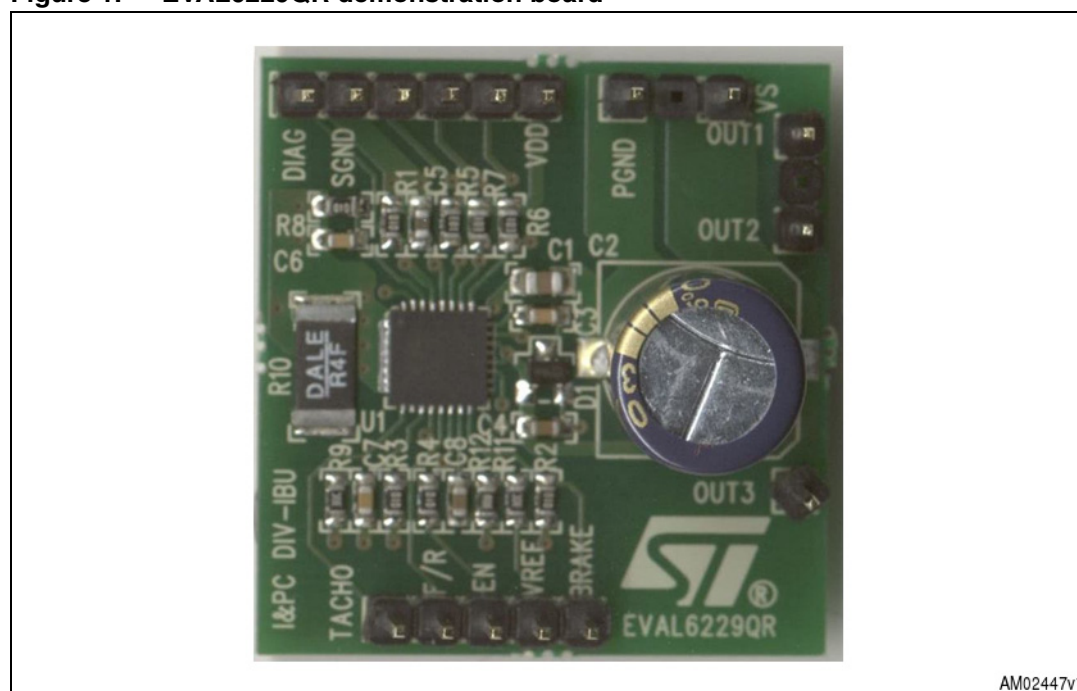
Figure 1. EVAL6229QR demonstration board
