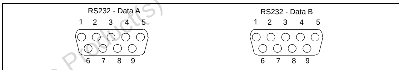
Figure 7: RS232 transmit and receive connectors: CN2, CN3
