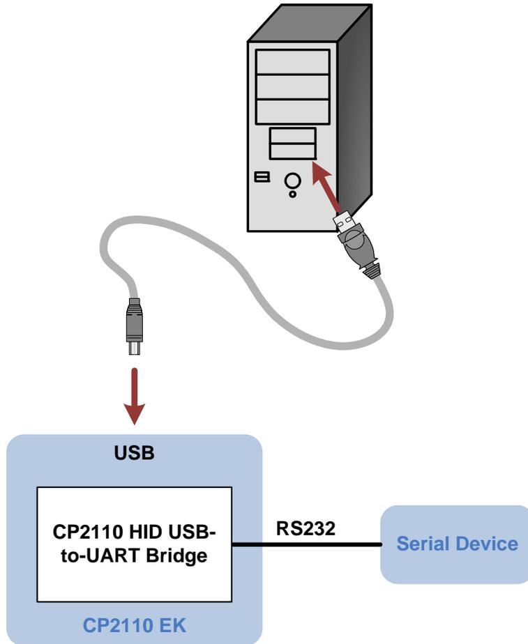
Figure 1. Hardware Setup
