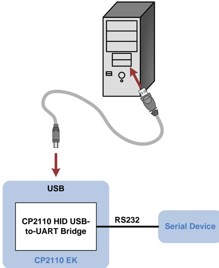
Figure 1. Hardware Setup
