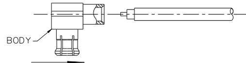
4. SOLDER CABLE CENTER CONDUCTOR TO CENTER CONTACT.
