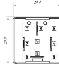
**Detail PCB version: minimum clearance requirements (see note below)**
