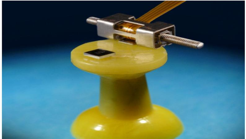
NSE-5310 position sensor – closed-loop kits include an NSE-5310 sensor. Evaluate the sensor and/or the performance of a closed-loop SQUIGGLE motor system.
