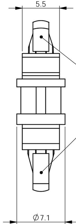
TO SNAP LOCK INTO A  $\text{Ø}4 \pm 0.08$  HOLE, INTO A 1.6 THICK PANEL, AT BOTH ENDS.
