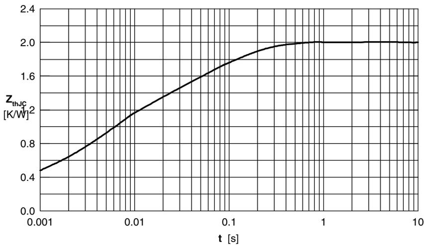
Fig. 6 Transient thermal impedance junction to case
