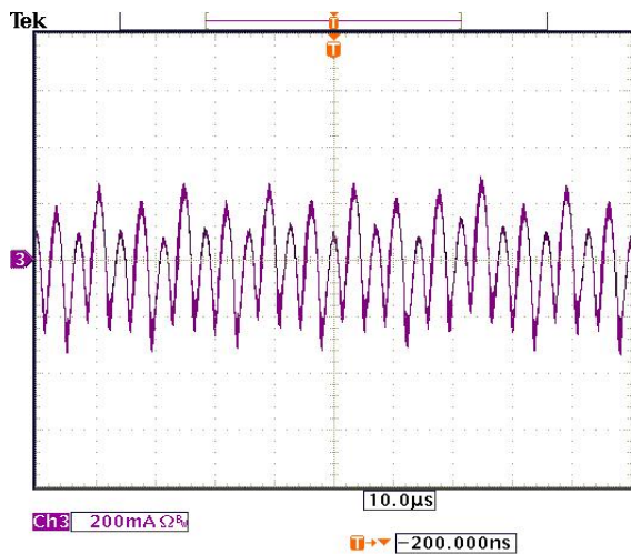
Figure 9: Input Terminal Ripple Current, i_c , at nominal input voltage and rated load current with 12\mu\text{H} source impedance and 150\mu\text{F} electrolytic capacitor (200 mA/div).
