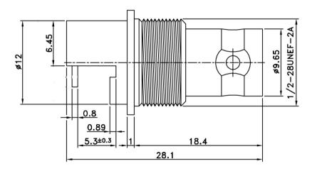
Body: Brass/Nickel Insulator: Teflon Pin: Brass/Gold
