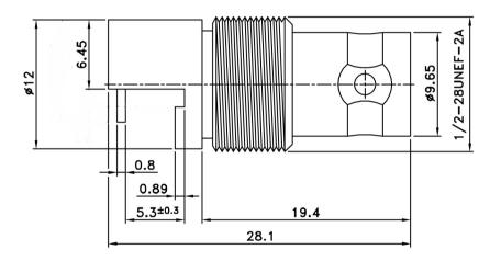
Body: Brass/Nickel Insulator: Teflon Pin: Brass/Gold
