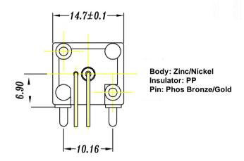
This is a basic dimensional drawing. If you require a more detailed drawing or if this connector does not fit your exact requirement please email - mailstop@bomarinterconnect.com or call 973-347-4040 for an alternate solution.
