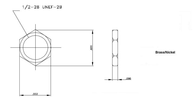
This is a basic dimensional drawing. If you require a more detailed drawing or if this connector does not fit your exact requirement please email - mailstop@bomarinterconnect.com or call 973-347-4040 for an alternate solution.
