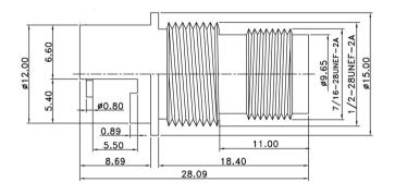
Body: Brass/Nickel Insulator: Teflon Pin: Brass/Gold
