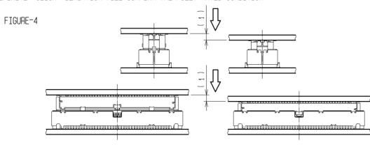
THE MATED CONDITIONS CAN BE RELEASED BY A DROP IMPACT. FIX THE CONNECTORS BY APPLYING PRESSURE IN THE MATING DIRECTION WITH THE DEVISE OR A BUFFER MATERIAL. **INOTES WHEN EXTRACTING**
