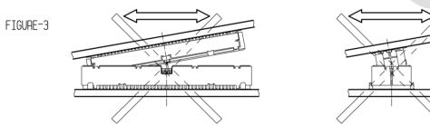
PRESS-DOWN EVENLY UNTIL SLIGHT RESISTANCE IS FELT. OVERCOMING THIS SLIGHT RESISTANCE WILL COMPLETE THE MATING OF RECEPTACLE WITH HEADER. A DEFINITE 'CLICK' SENSATION WILL CONFIRM THE FULLY MATED CONDITION.
