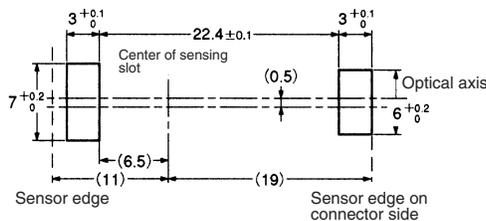
The Photomicrosensor can be mounted to 0.8- to 1.6-mm-thick panels.
