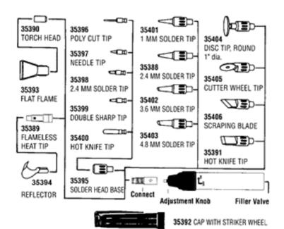
35407 POPULAR ACCESSORY KIT INCLUDES: 35395 SOLDER HEAD BASE, 35396 POLY CUT TIP, 35397 NEEDLE TIP, 35398 2.4 MM SOLDER TIP, 35399 DOUBLE SHARP TIP, 35400 HOT KNIFE TIP
