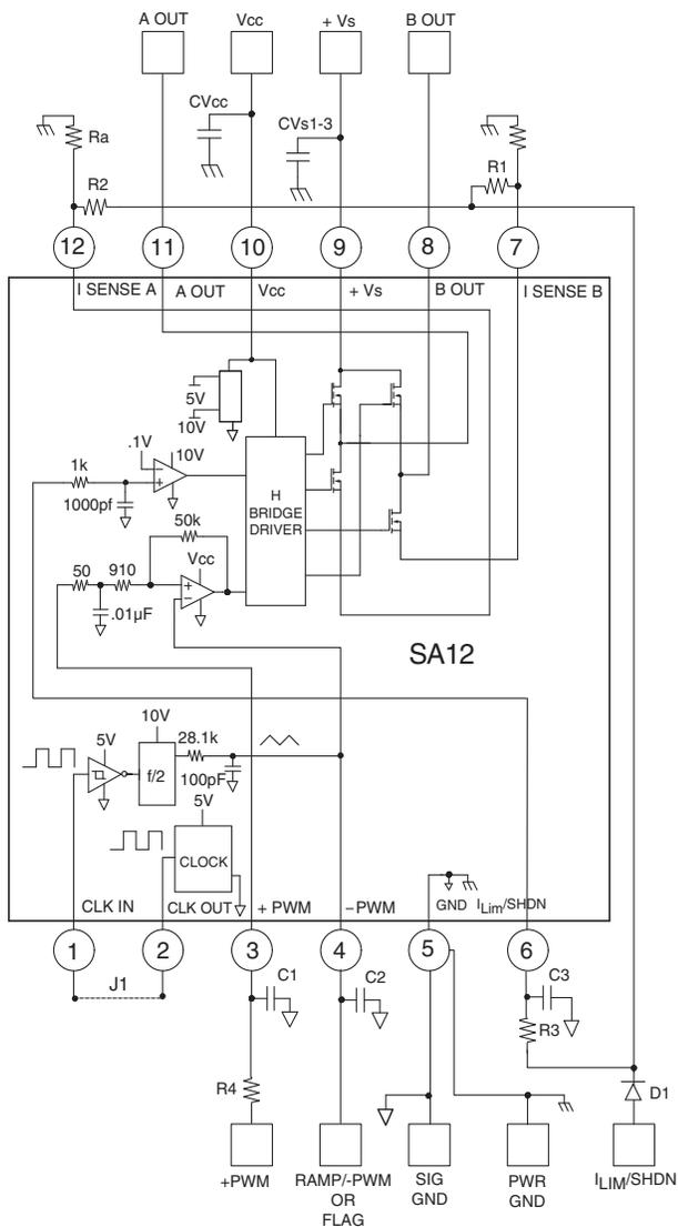
The schematic of Figure 4 can be used to verify the functionality of your amplifier and help you gain a familiarity with proper operation. At either A Out or B Out, with respect to ground, you should observe a square wave approximately 30 V in amplitude with a fixed frequency and duty cycle that varies from approximately 0 to 100% at a rate of 1 Hz. The current limit is set to 10 amps.
