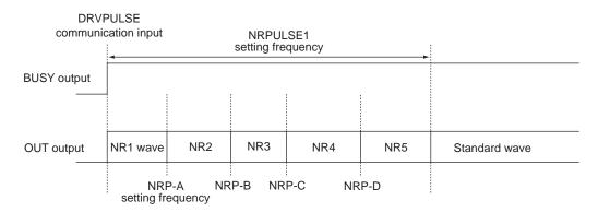
If, as an example, the NRPULSE1 setting is set to 15, the NRP-A setting is set to 3, the NRP-B setting is set to 6, the NRP-C setting is set to 9 and the NRP-D setting is set to 12, then after the NR1 waveform is output for three periods, the NR2 waveform for three periods, the NR3 waveform for three periods and the NR5 waveform for three periods, the standard waveform is output for a period equivalent to the STP x DRVPULSE period.
