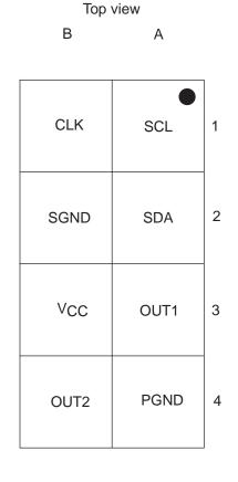
A1:CLK B1:CLK A2:SDA B2:SGND A3:OUT1 B3:VCC A4:PGND B4:OUT2
