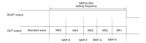
During the fall-time operation, the waveforms are output in sequence from the NR5 waveform to the NR1 waveform. The method used to set the switching timing is the same as for the rise-time operation.
