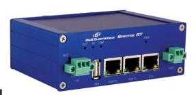
The SPECTRE RT industrial router connects Ethernet equipment in tough environments where office-grade equipment can't handle the job. With Ethernet, USB, I/O and auxiliary ports it's a flexible device with the built-in ability to handle multiple data communications protocols and to fit into virtually any network topology.
