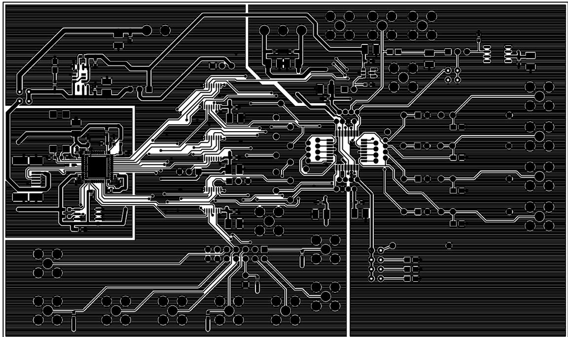
Figure 8. Solder Side PCB Drawing
