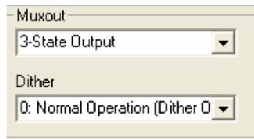
In both cases you will need to update the Register 6 and Register 2 after the dither mode has been selected. Register 2 is updated as a different phase values is used for dither off and on. The software will load Dither Off as default.
