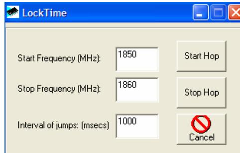
Enter start ,stop frequencies and interval of the jump in milliseconds and then click on the “start hop”. To stop the hopping click on the “stop” and then “cancel” to return to the main form. As the ADF4193 is writing to phase registers before it writes the frequency information there will be more than one LE pulse for each frequency write.
