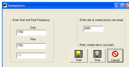
Start and stop frequencies are entered with the rate of sweep in milliseconds. The resolution of the sweep is taken from the channel already set on the main form and shown underneath the “stop” display
