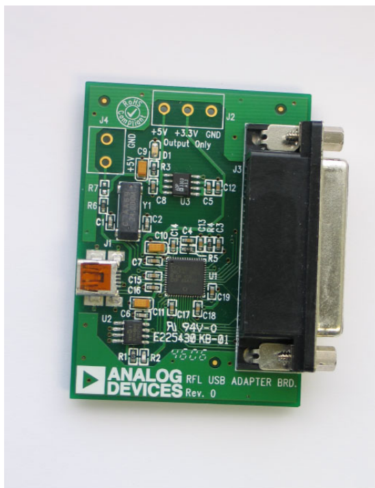
Figure 1. EVAL-ADF4XXXZ-USB Adapter Board
