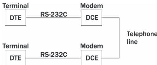
*Note: In many applications, DCEs are unnecessary. This allows you to use a null modem cable (modem eliminator cable) to directly connect two DTE-type devices.*
