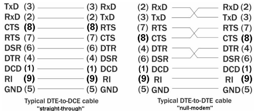
Quatech Serial Adapters are DTE devices that connect to peripheral equipment through a male DB-9 connector. The following table lists the serial port connector definitions.
