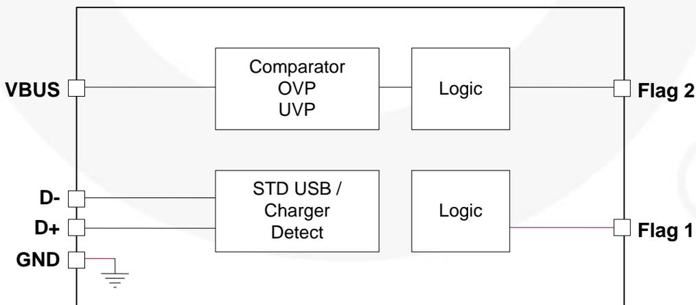
Figure 1. Block Diagram
