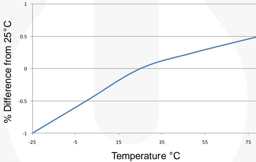
Figure 13. VReference ( $V_{REF}$ ) vs. Temperature
