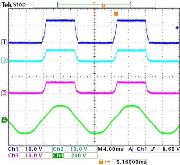
Ch1:  $V_{Line}$  (Pin 3), 10V/Div
