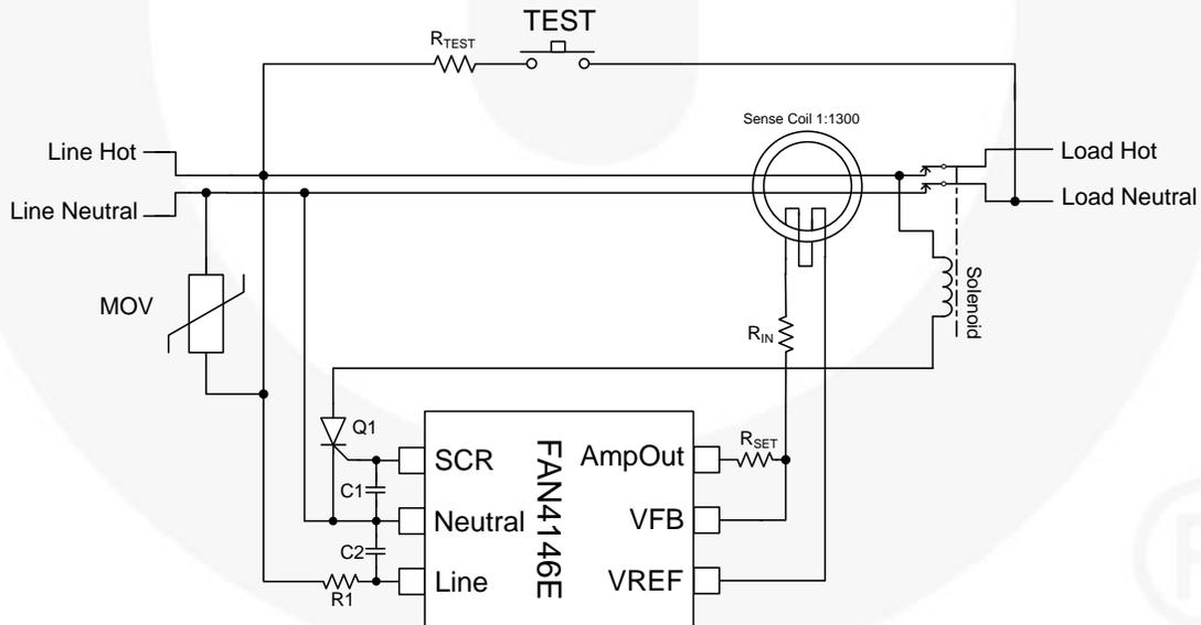
Figure 2. 220V<sub>AC</sub> RCD Application<sup>(4)</sup>
