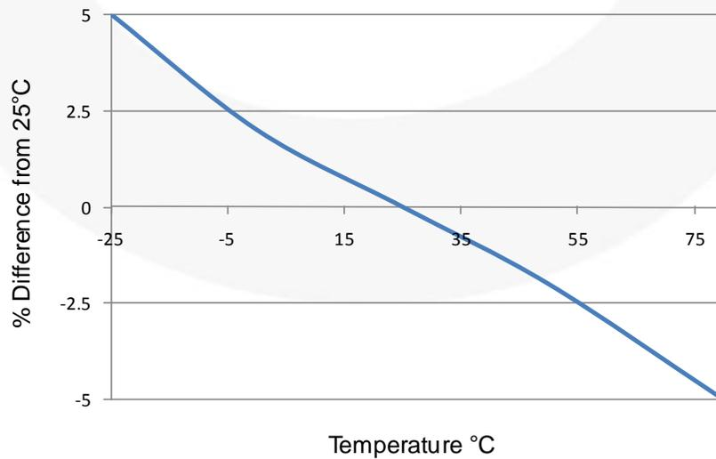
Figure 14. SCR Output Current ( $I_{OUT}$ ) vs. Temperature
