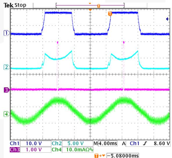
Ch1:  $V_{Line}$  (Pin 3), 10V/Div
