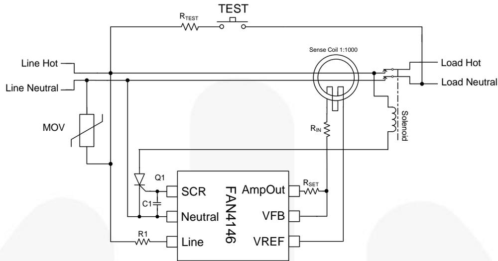
Figure 1. 120/220V<sub>AC</sub> ALCI Application<sup>(2)</sup>
