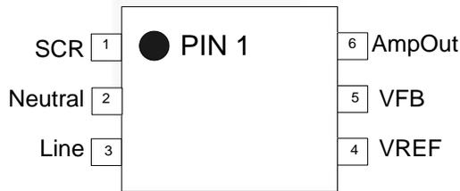
Figure 4. Pin Configuration
