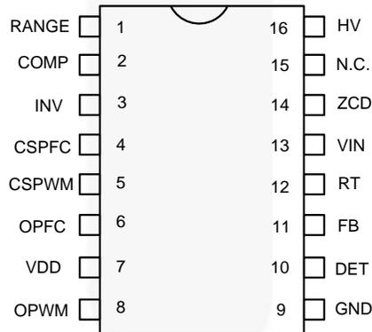
Figure 4. Pin Configuration
