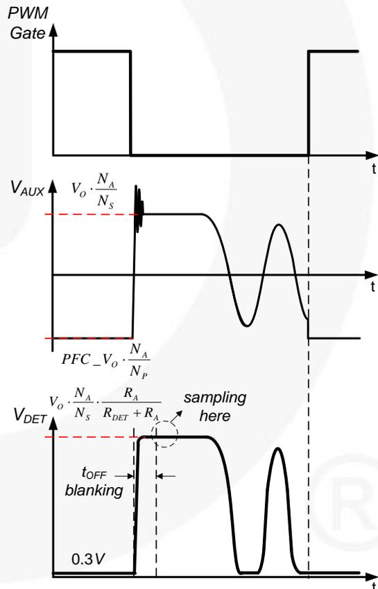
Figure 44. Operation Waveform of Output Over-Voltage Detection
