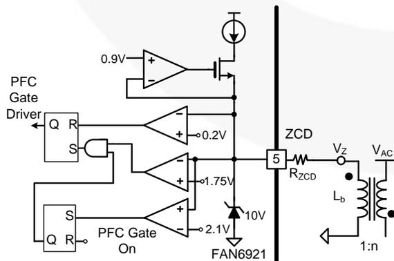
**Figure 30. Internal Block of the Zero-Current Detection**
