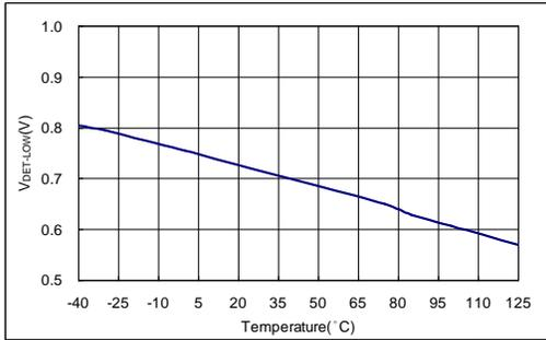
**Figure 21. Lower Clamp Voltage of DET Pin**
