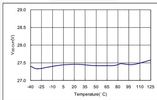
**Figure 8. V<sub>DD</sub> Over-Voltage Protection Threshold**
