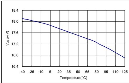
**Figure 5. Turn-On Threshold Voltage**
