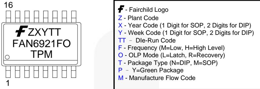
Figure 3. Marking Diagram
