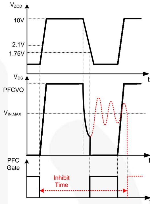
**Figure 31. Operation Waveforms of PFC Zero-Current Detection**
