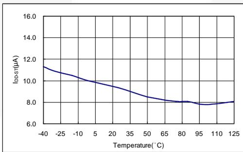
**Figure 9. Startup Current**
