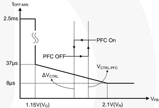
Figure 38.  $V_{FB}$  Voltage vs.  $t_{OFF-MIN}$  Time Characteristic Curve
