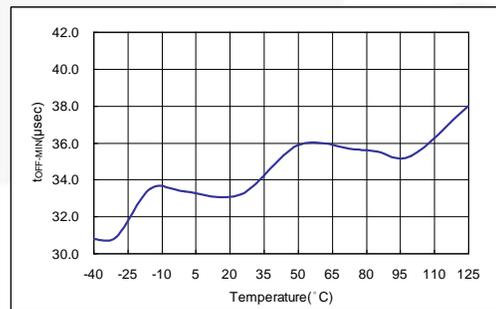
Figure 20. PWM Minimum Off Time for  $V_{FB} = V_G$
