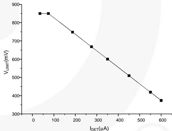
**Figure 42.  $I_{DET}$  Current vs.  $V_{LIMIT}$  Voltage Characteristic Curve**
