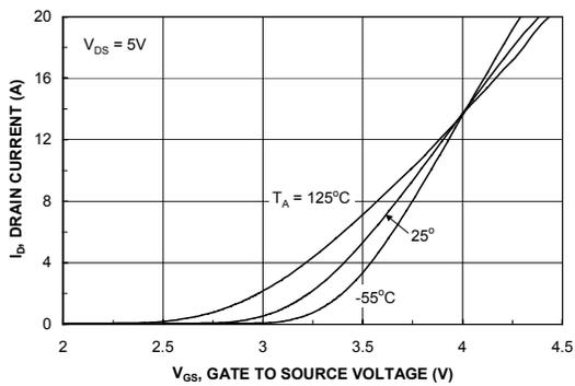
Figure 5. Transfer Characteristics.
