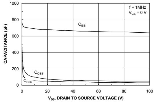
Figure 8. Capacitance Characteristics.
