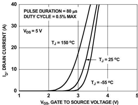
**Figure 5. Transfer Characteristics**
