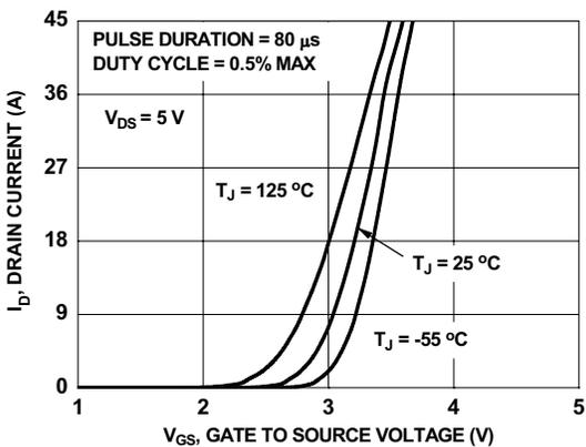
**Figure 5. Transfer Characteristics**
