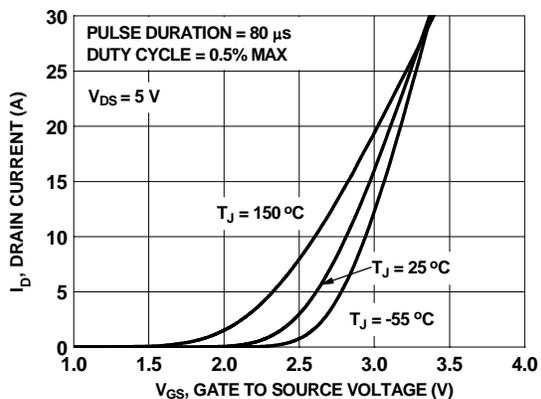
Figure 5. Transfer Characteristics
