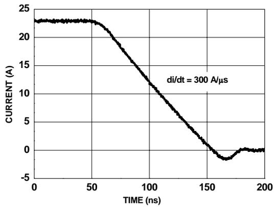
Figure 14. FDMS7572S SyncFET body diode reverse recovery characteristic
