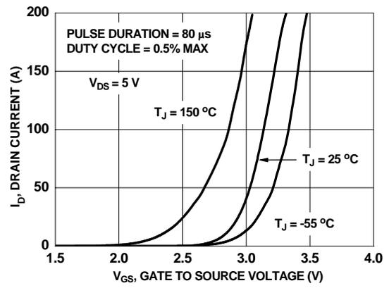
**Figure 5. Transfer Characteristics**
